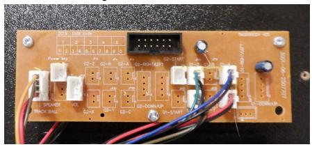
4. Remove the 3 screws from the printed circuit board. The PCB will now be unattached to the frame.
