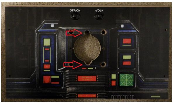
8. Use a coping saw or other similar saw to cut the circular hole into a rectangular hole. Notice there is a black square around the large hole where there are no graphics. The left and right side should be cut on the edges of this square outline. The top and bottom should be cut leaving about 1/2" of material between the large hole and the 4 main mounting holes as shown below. The cut does not need to be perfect as it will be covered by the controller and not visible after final assembly.
