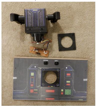
6. Drill out the 4 mounting holes with a 7/16 drill bit.
