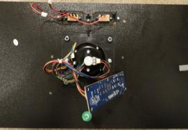
5. Remove 4 screws from the top of the control panel that holds the yoke to the panel. The 4 screws are hidden by the yoke. The yoke must be turned at an angle to gain access to the screws.
