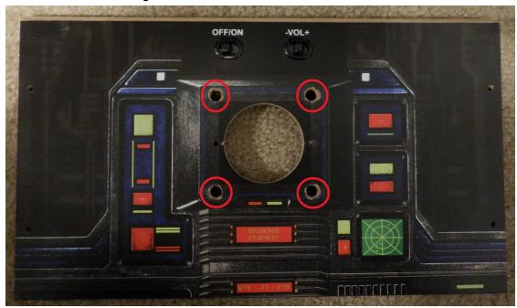
7. Drill a hole at the top and on the bottom of the large opening using a 1/2 drill bit. These holes will allow the pair of nuts on the bottom of the yoke to mount below the surface of the control panel.
